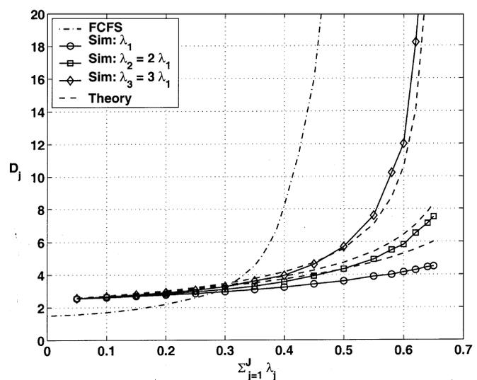
Fig. 4. BNDMA: Delay versus total load.
