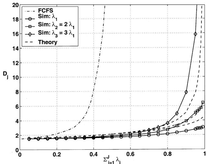
Fig. 2. NDMA: Delay versus total load.
