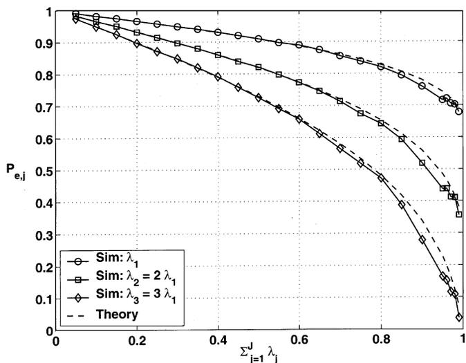
Fig. 1. NDMA:  $P_{e,j}$  versus total load.
