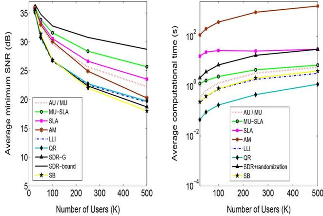
Fig. 2. Comparison of average minimum SNR and computation time versus  $K$  for  $N = 20$  antennas when the user channels are drawn from an i.i.d. Gaussian distribution.
