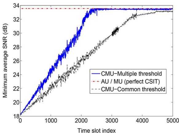
Fig. 9. Average minimum SNR of CMU algorithm for  $N = 20$ ,  $K = 50$ .
