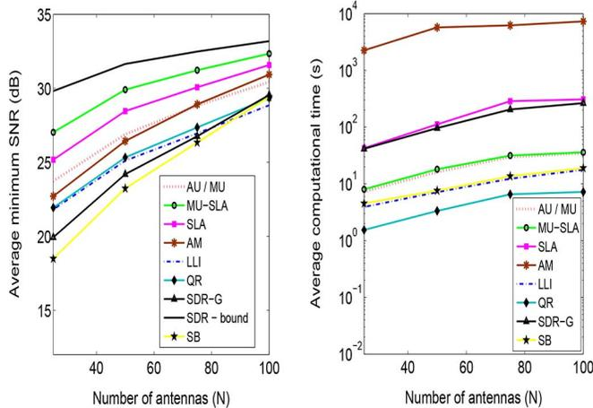
Fig. 3. Comparison of average minimum SNR and computation time versus  $N$  for  $K = 450$  users when the user channels are drawn from an i.i.d. Gaussian distribution.
