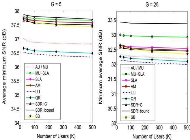
Fig. 4. Comparison of average minimum SNR versus  $K$  for  $N = 20$  antennas when channels to all users are drawn from a mixture of  $G = 5$  (left) and  $G = 25$  (right) Rician distributions.
