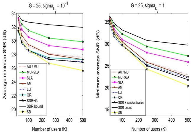
Fig. 5. Comparison of average minimum SNR versus  $K$  for  $N = 20$  antennas when channels to all users are drawn from a mixture of  $G = 25$  Rician distributions with  $\sigma_{k_g} = 10^{-1}$  (left) and  $\sigma_{k_g} = 1$  (right).
