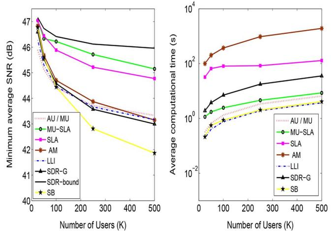
Fig. 6. Comparison of average minimum SNR and computation time versus  $K$  for  $N = 20$  antennas, when  $\{\mathbf{R}_k\}_{k=1}^K$  are full rank.
