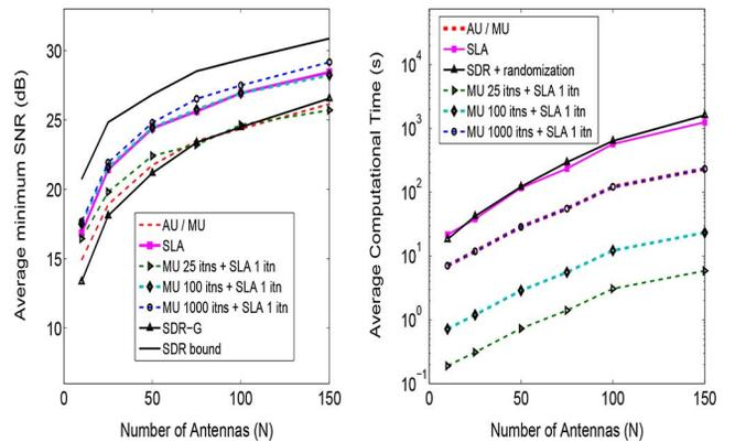
Fig. 7. Comparison of minimum average SNR and computation time versus  $N$  for  $K = 500$  users, when channels to all users are drawn from an i.i.d. complex Gaussian distribution.
