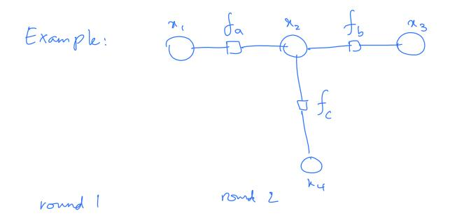
$M_{1a}(x_{1}) = ( P_{a2}(x_{2}) = \sum_{x_{1}} f_{a}(x_{1})x_{2})P_{1a}(x_{1})$   $P_{4c}(x_{4}) = ( P_{b2}(x_{2}) = \sum_{x_{3}} f_{b}(x_{3})x_{2})P_{3b}(x_{3})$   $P_{3b}(x_{3}) = ( P_{c2}(x_{2}) = \sum_{x_{4}} f_{c}(x_{2})x_{4})P_{4c}(x_{4})$
